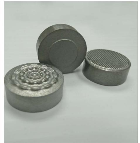
*RockStorm technology was selected to overcome bit failure challenges with its superior wear and impact resistance, enabled by a proprietary diamond grain-size distribution and engineered tungsten carbide substrate.*
