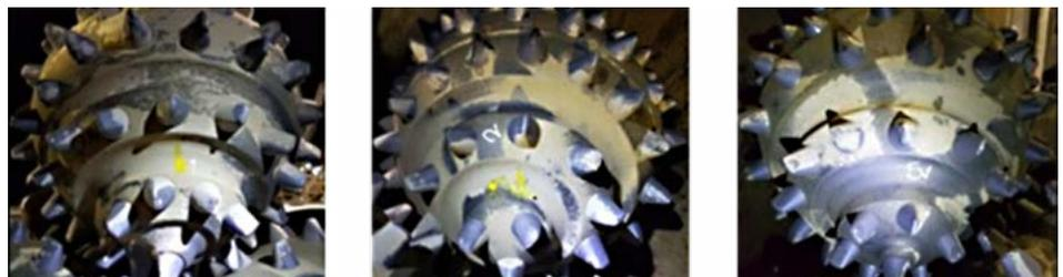
*After reaching TD, the Xplorer bit was pulled out of hole, and the dull condition on the bit was in good condition.*
