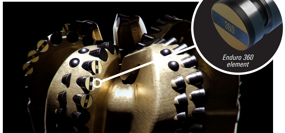
Rolling diamond element cutters are positioned in the high-wear shoulder area to improve EnduroBlade 360 bit durability. As the cutting element rotates 360°, wear is evenly distributed around the perimeter of the diamond table.
