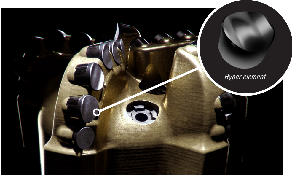
The hyperbolic shape of the Hyper element mitigates the severe bit balling that commonly occurs with flat PDC cutters by creating small cuttings chips, improving cuttings removal and increasing ROP.
