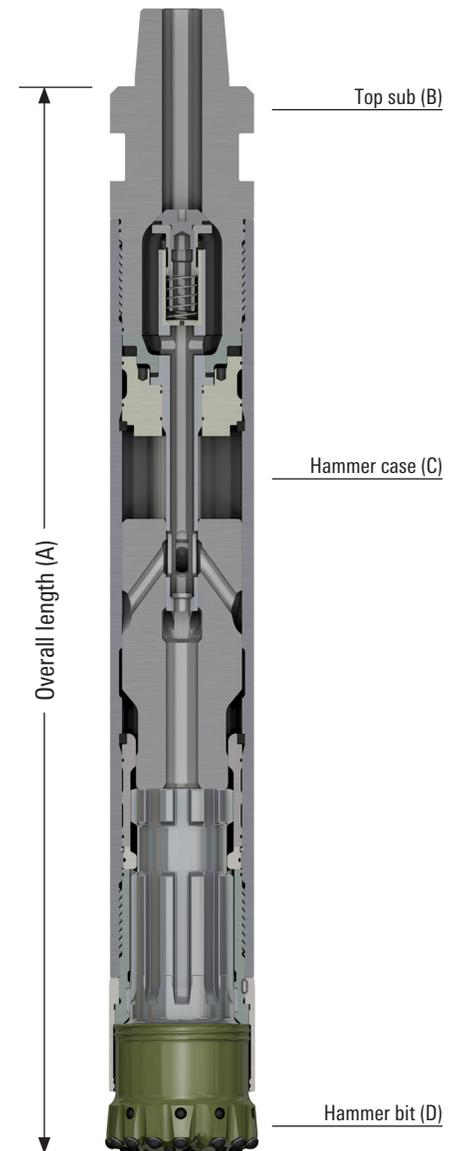
The 12-in Impax hammer system's integral steel valve design increases the hammer's resistance to failure from high temperature or erosion from water.
