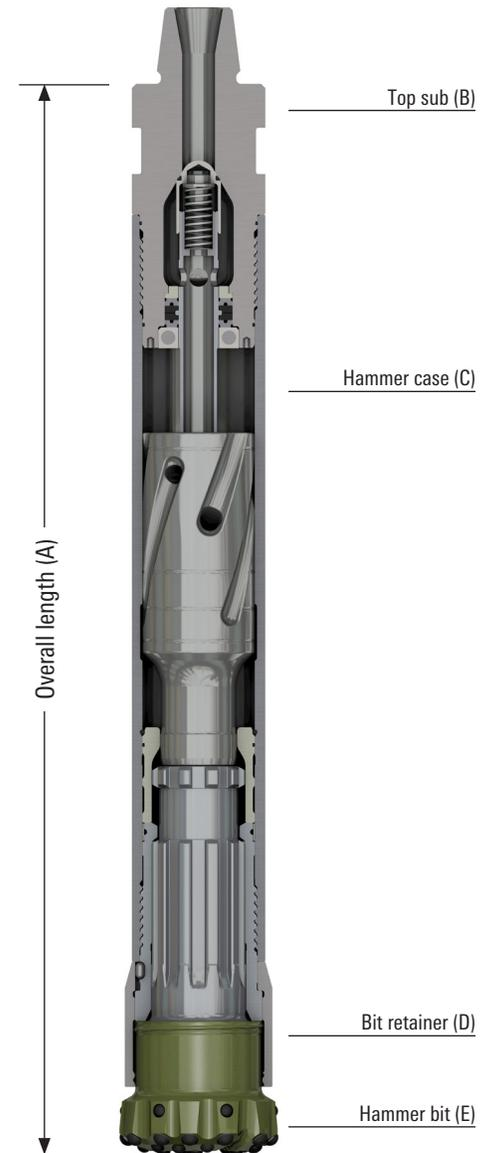
*The 8-in Impax hammer system has a floating feed tube to ensure the piston and feed tube are in proper alignment, which reduces wear and risk of premature failure.*
