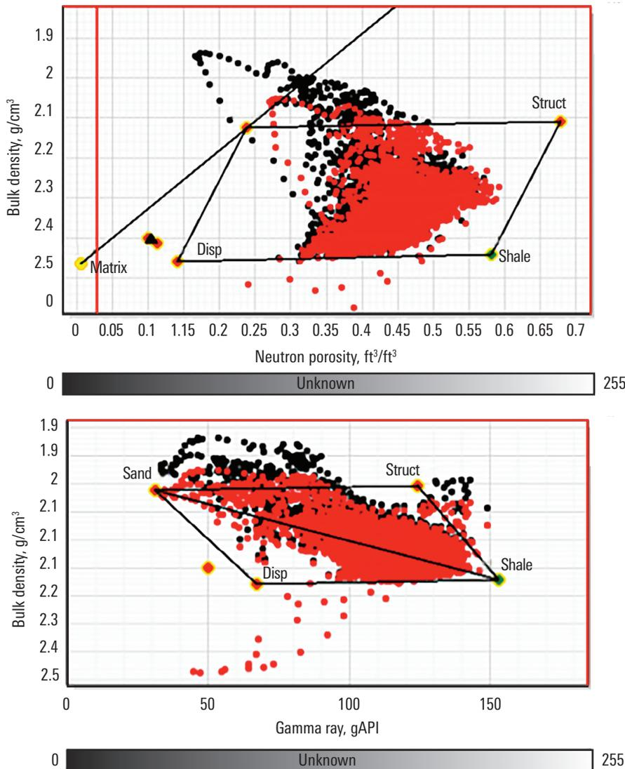
The red points on crossplots of bulk density versus neutron porosity (top) and gamma ray (bottom) are corrected for hydrocarbon effects to determine four fractions of laminated shaly sands.
