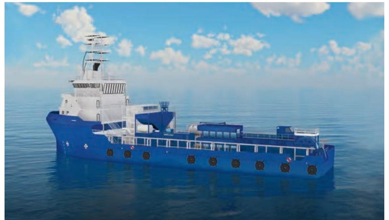
The FlexSTIM Pronto modular design allows equipment installation in 7 days on a standard Bourbon GPA 670 vessel.
