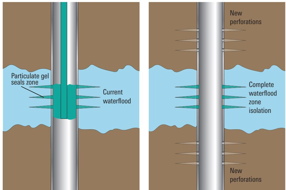
Coiled tubing delivered the particulate gel to the watered-out zone and squeezed until the perforations were sealed. New perforations were then shot above and below the plugged zone to enable further oil production.
