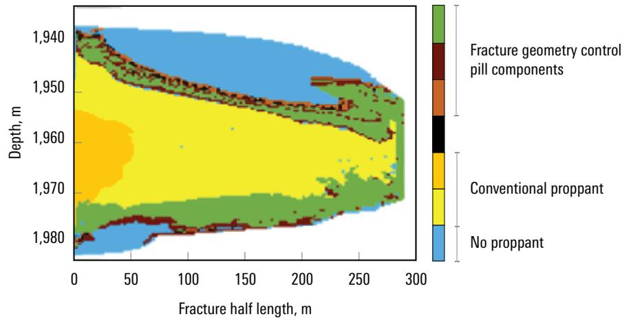
The BroadBand Shield service design for Well MA6 created low-permeability layers at the bottom and top of the fracture to limit height growth into water zones and to minimize permeability at the edges of the fracture—hindering the progress of any water that might reach it.
