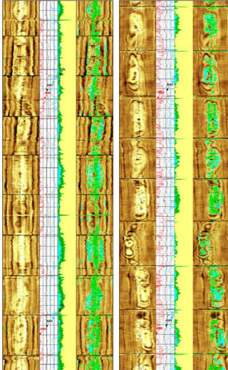
*In one of the conventionally cemented wells, left, the cement bond is mostly acceptable; however, a long and continuous channel exists and could carry fracturing fluid between perforation clusters. In a well cemented with Fulcrum technology, the cement bond is improved, and the small channels are not connected, so fracturing fluid cannot migrate very far.*
