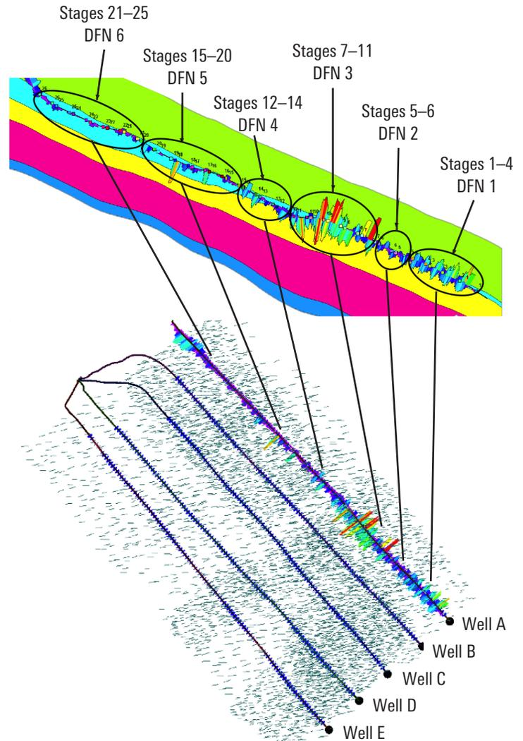
*Discrete fracture network model sets for characterizing reservoir heterogeneity along the lateral complex hydraulic fracture geometry using the UFM model.*
