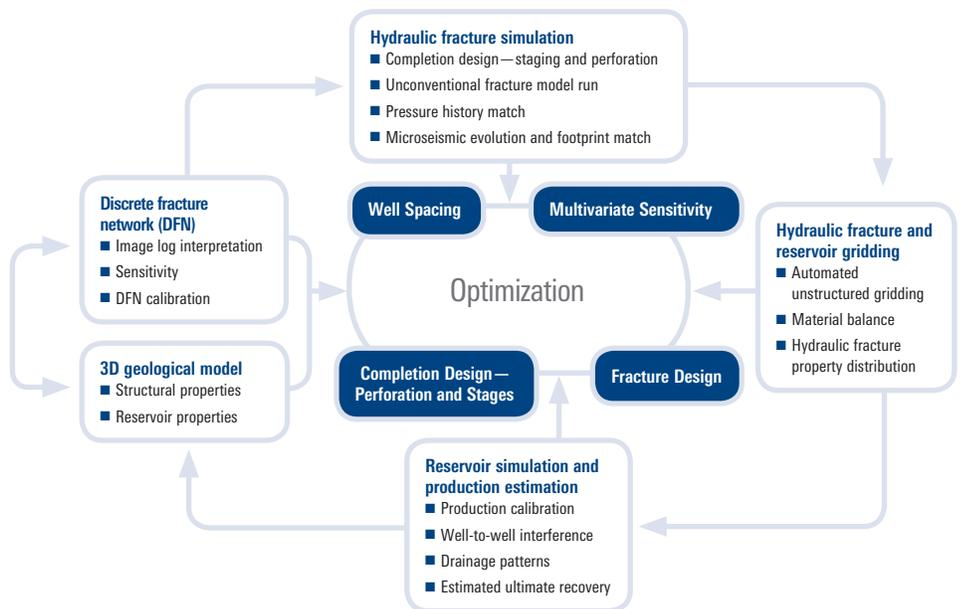
*Integrated multiwell completion workflow using Kinetix Shale software.*
