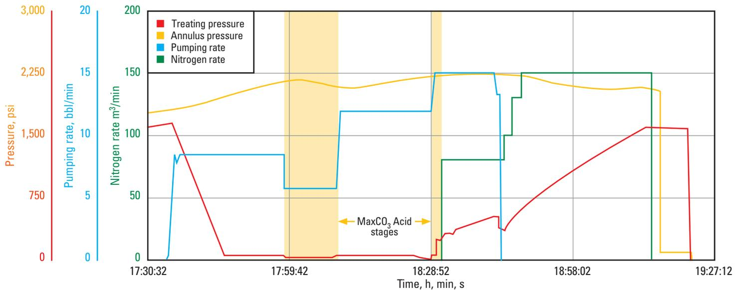
Treatment plot of MaxCO<sub>3</sub> Acid system showing diverter stages (shaded orange). The treatment pressure was difficult to maintain at the start of the treatment, but increased significantly following the second MaxCO<sub>3</sub> Acid stage.
