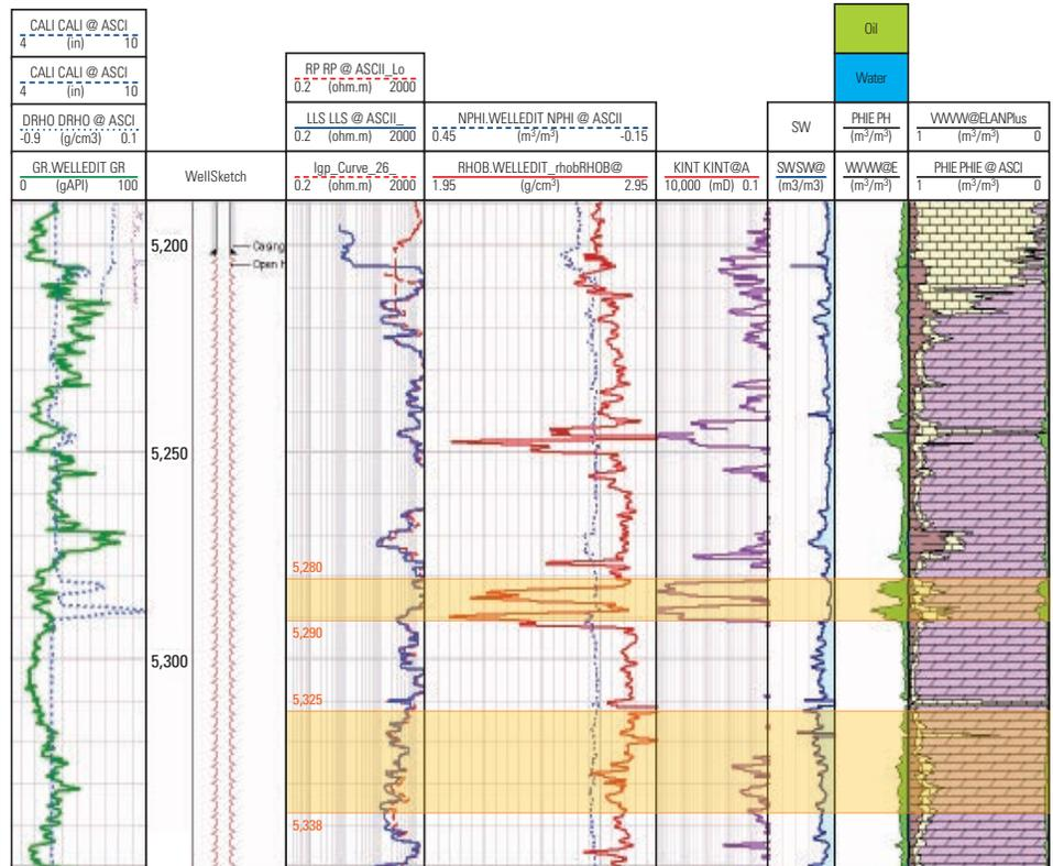
Well logs identifying the two target zones. The upper zone has a permeability of over 1D, indicating natural fractures. The lower zone has an average matrix permeability of approximately 3 mD. Such large contrasts make effective uniform stimulation challenging.
