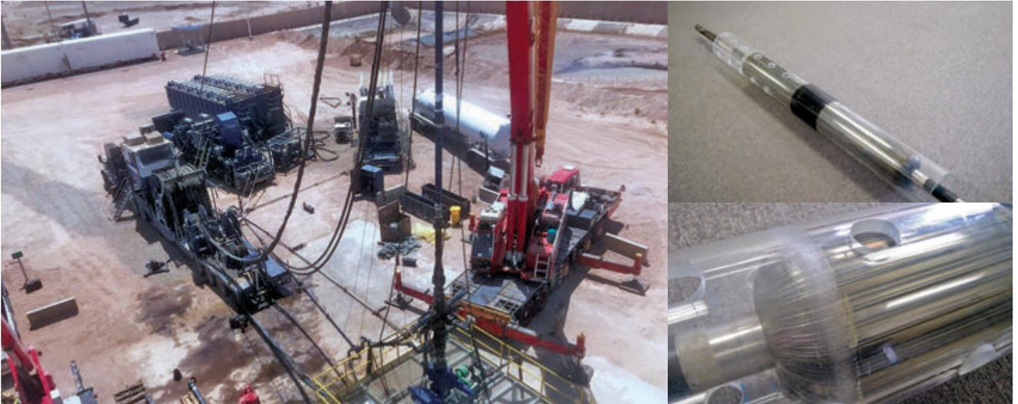
*A CoilFLATE packer (right) isolated the high-permeability zones, enabling the OpenPath Reach service to precisely stimulate lower-permeability zones using less fluid and equipment compared with conventional emulsified acid stimulation.*
