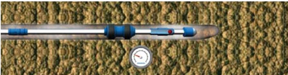
*The mechanical openhole packer with tandem elements is rated to 68.9 MPa [10,000 psi] and 218 degC [425 degF].*
