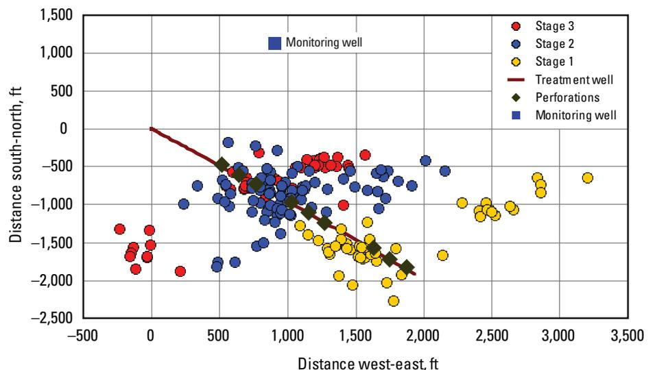
Map view of microseismic events from a three-stage slickwater ClearFRAC\* LT low-temperature polymer-free stimulation treatment.
