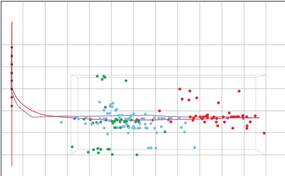
*Transverse view of microseismic locations from a three-stage slickwater ClearFRAC LT stimulation treatment orthogonal to the preferred fracture orientation. Color-coding indicates which of the three seismic events is responsible for each location.*
