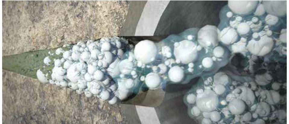
*An engineered composite fluid of degradable particles and fibers temporarily isolates fractures at the wellbore.*
