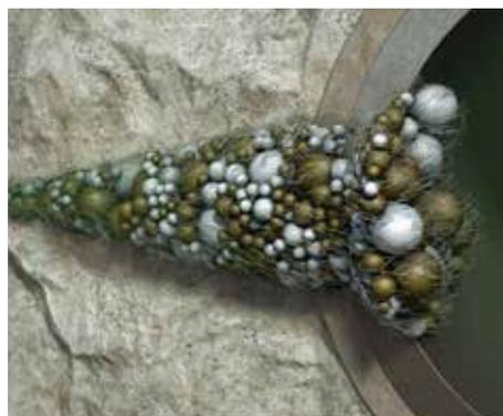
*Enhanced-conductivity partially degradable composite pill.*
