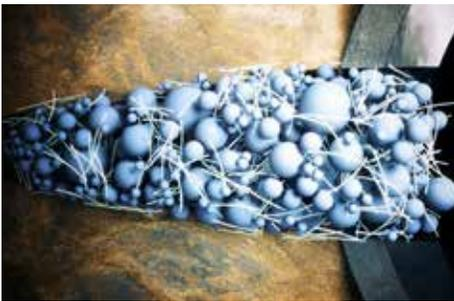
*The ultralow-temperature diversion pill improves flexibility and reliability in formations with temperatures as low as 70 degF.*
