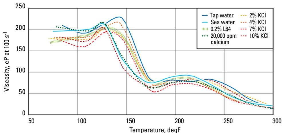
The ClearFRAC XT system exhibits excellent proppant transport at low surfactant concentrations and low viscosity.
