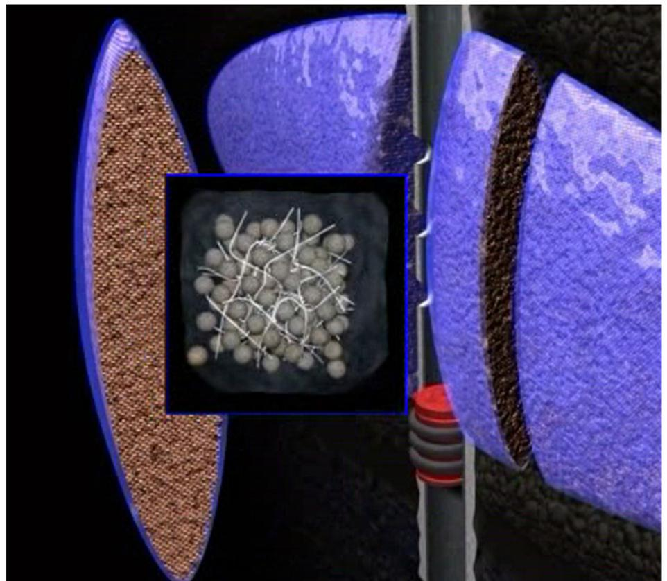
*Fiber-based mechanical support for proppant pack.*
