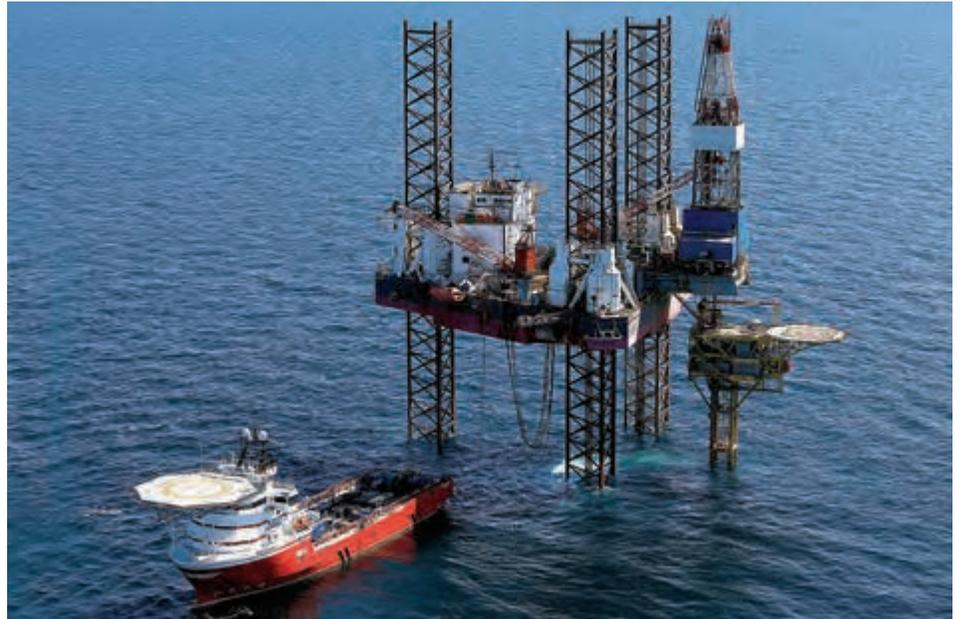
*The FlexSTIM system turns a standard supply vessel into a powerful, high-capacity stimulation platform.*
