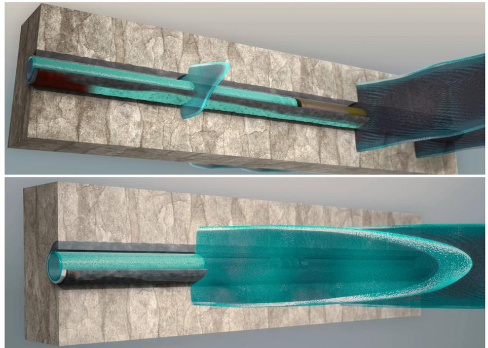
*Fulcrum technology improves fracturing performance by reacting with NAF to limit its mobility and improve resistance to out-of-zone fracturing fluid flow. Top, fracturing fluid migrates between stages behind the casing through mud channels, resulting in stunted fracture extension. Bottom, Fulcrum technology reduces mud channel permeability and mobility, keep the fracturing fluid in the intended stage to improve fracture length and efficiency.*
