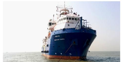
*To perform efficient stimulation and well testing operations, the pumps on Greatship Ramya deliver up to 8,000 hhp with a variety of configurations to enable flexibility in rates and pressures.*
