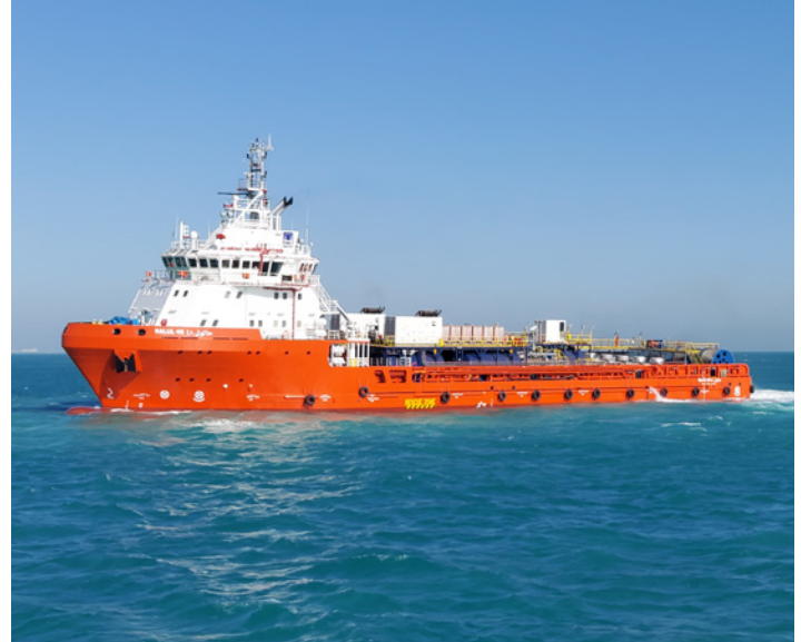
The Halul-48 well stimulation vessel equipped with second-generation FlexSTIM system.
