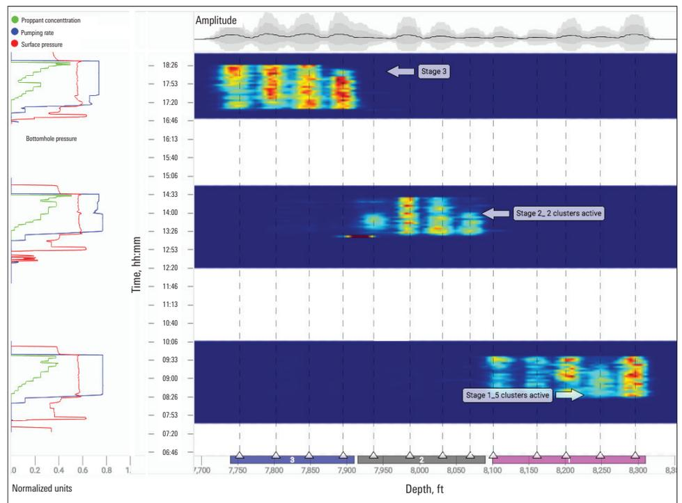
*Kinetix RT software is used to monitor perforation activity during two fracturing stages with hDVS from permanent fiber optic installed behind the casing.*
