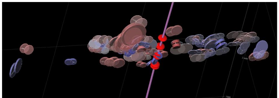
A unique and intuitive display of moment tensor results represents the source mechanisms for one stage of microseismic events in an expansion, opening, and slip (EOS) glyph.
