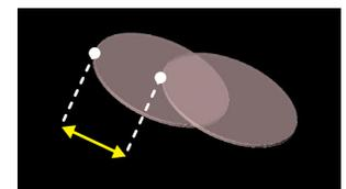
Slip in the fracture plane is depicted by the orientation of the disks and the displacement between disk centers.
