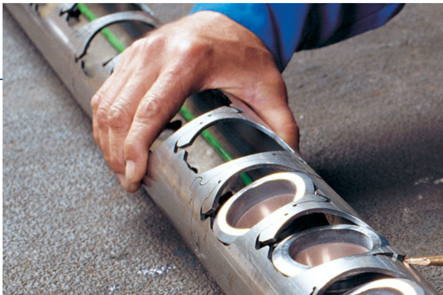
The OrientXact* perforating system is an important component of the perforation optimization part of the PowerSTIM process.
