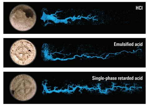
The performance of the single-phase retarded acid is similar to that of an emulsified acid and much better than HCl in core flow experiments at 275 degF [135 degC] in 8-mD Indiana limestone cores with equal amount of acid injected into the cores at equal rates. The wormhole from HCl penetrates only half of the core, while the wormholes from the single-phase retarded acid and the emulsified acid extend the entire length.
