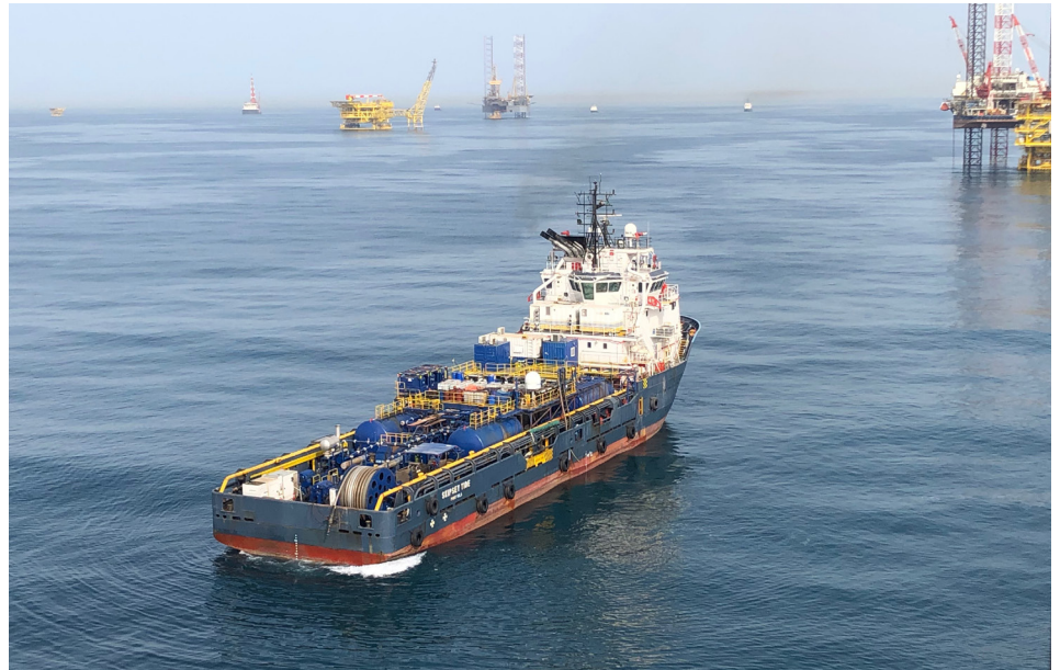
For offshore stimulation, the Skipsey Tide vessel delivers acid and other fluids with pumps that deliver up to 6,650 hhp.
