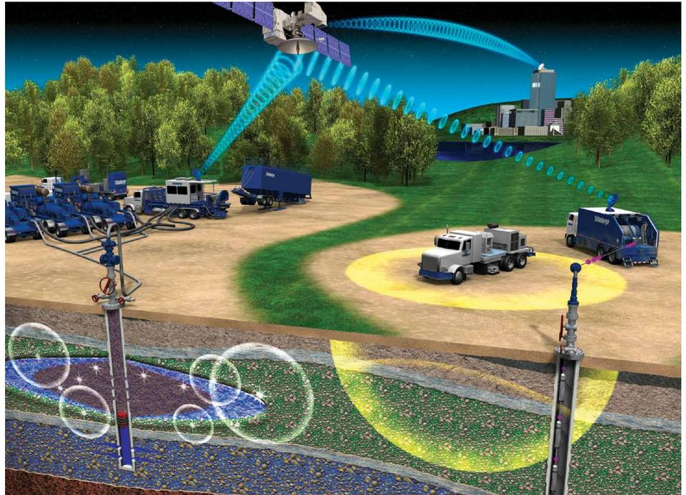
*Computer-generated illustration of a hydraulic fracture creating microseisms (mini-earthquakes) that are detected and located by the VSI\* versatile seismic imager tool in an observation well.*
