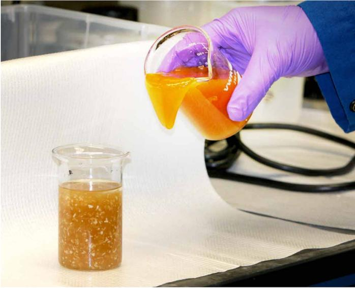
*xWATER service was used to create a high-performance crosslinked gel using 100% produced water (fluid on right) with concentrations of 280,000 mg/L total dissolved solids, 25,000 mg/L hardness, and 60 mg/L boron. With the same waters, the failure of a traditional fluid system (fluid on left) is evident, showing an unstable fluid with visible scale.*
