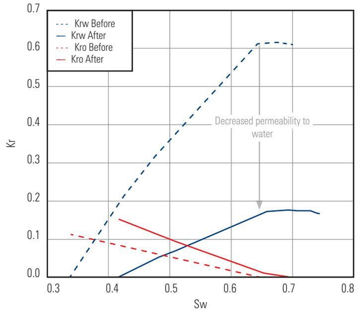
As indicated in this graph, the ZONETROL XT system reduces the relative permeability of the reservoir to water by up to 75% with little if any change in the permeability of the reservoir to oil.
