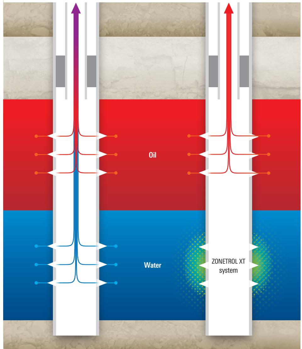
*Using the ZONETROL XT system, right, reduces permeability to water while maintaining permeability to oil.*
