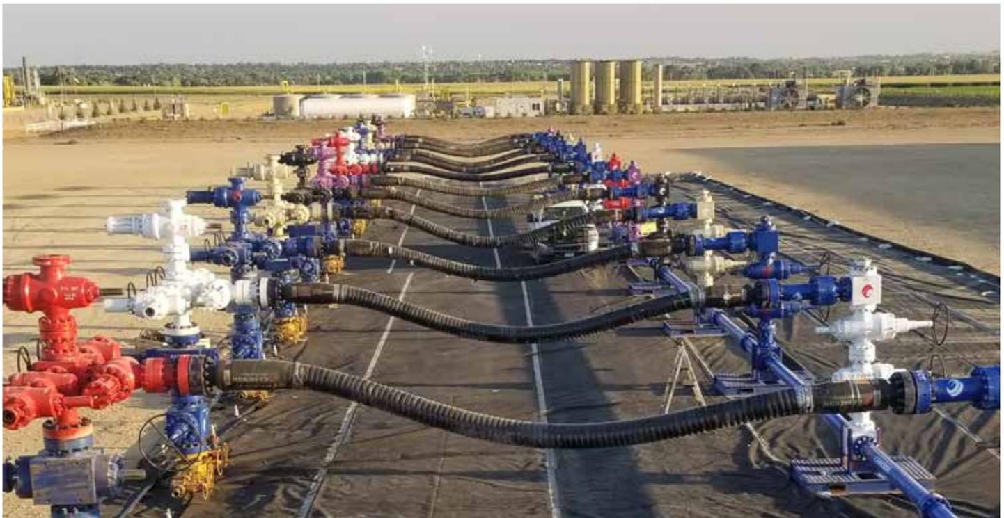
*MonoFlex technology helped PDC Energy cut iron-related NPT during zipper frac operations by eliminating more than 200 pieces of frac iron and their connections—each one a potential leak path.*
