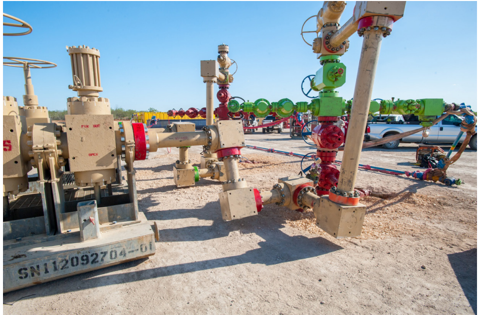
The Monoline technology, consisting of high-pressure pipe segments joined with 90° elbows and swivel flanges, eliminated multiple connectors.
