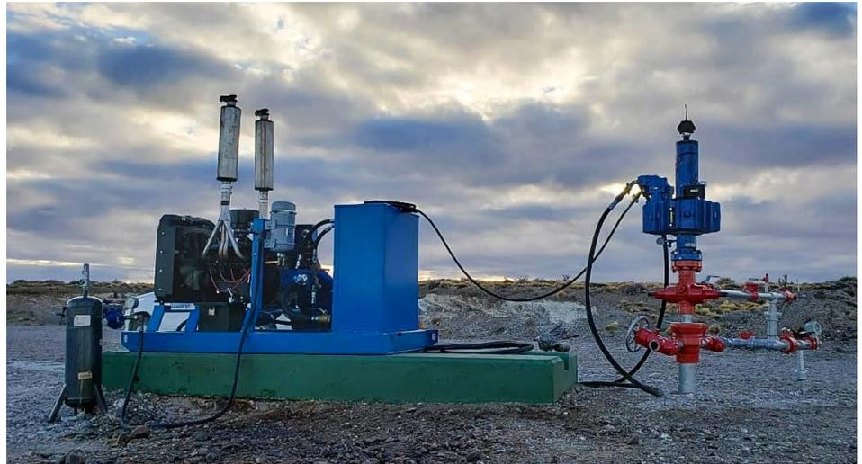
*The hydraulic drivehead with torque control has eliminated sucker rod failures, and the absence of exposed moving parts near the wellhead has enhanced safety.*
