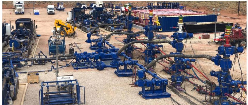
The 5-in MonoFlex technology is a flexible way to simplify fracturing fluid delivery with a clean wellsite footprint.
