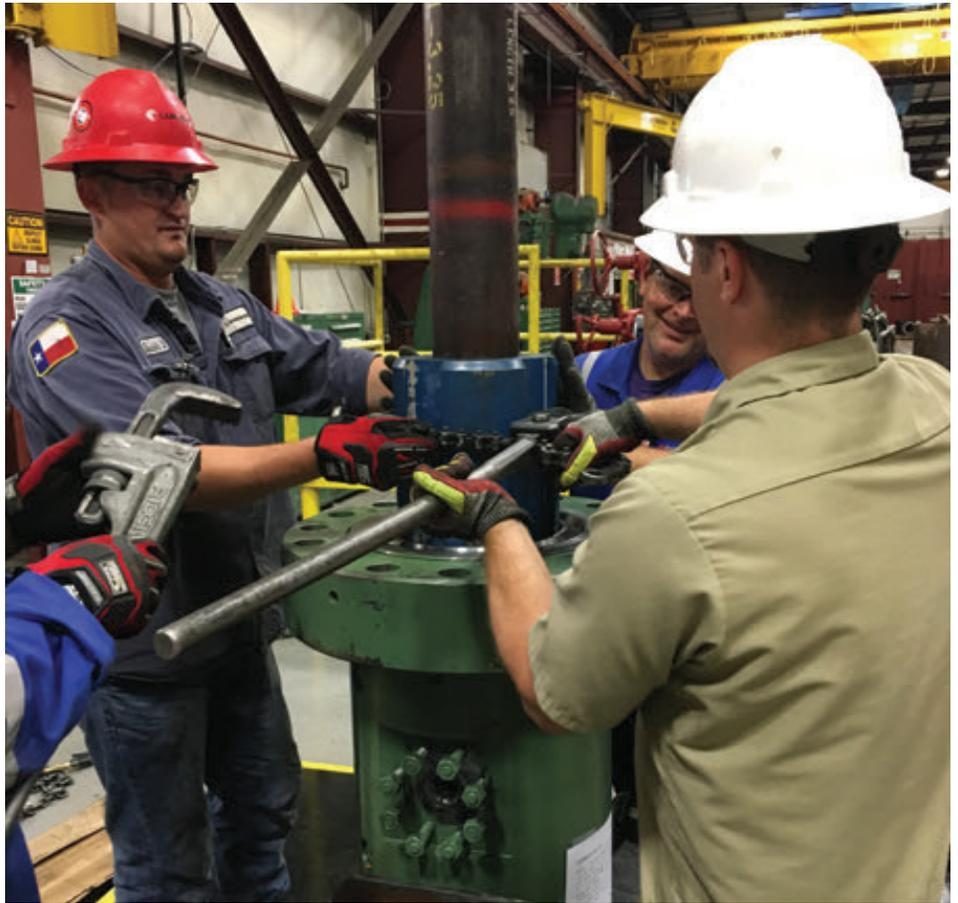
*Cameron personnel are performing a stackup test on an SSD-II wellhead system.*
