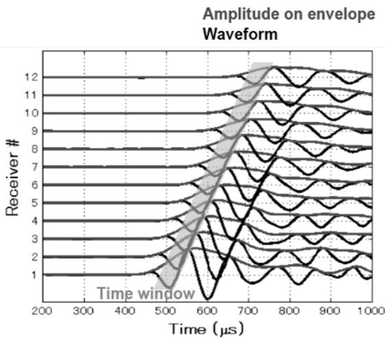
Figure 2: Early arrival detection for amplitude and attenuation through the receiver array
