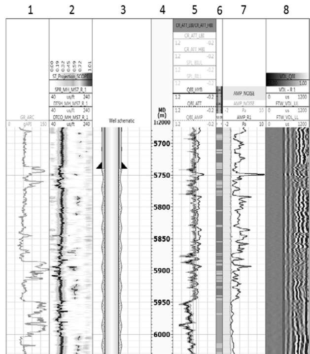
Figure 8: A log excerpt showing the hybrid bond index result and associated quality control indicators.
