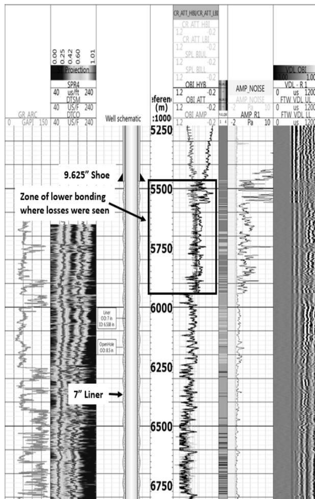
Figure 9: Zone of lost circulation correlated with low hybrid cement bond index values. A lack of good cement bonding was the reason the initial pressure test failed. The open-hole monopole data is shown for reference.
