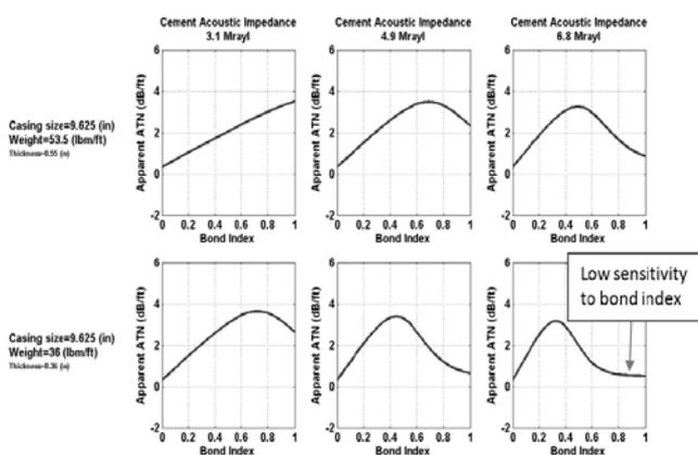
Figure 4: Modeled apparent attenuation vs. bond index for a 6.75-in. tool inside 9.625-in. casing.
