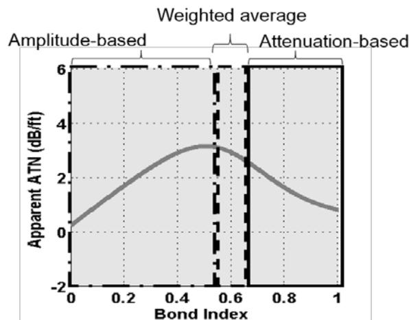
Figure 6: A modeled apparent attenuation vs. bond index curve is shown to illustrate where amplitude and attenuation based methods would be applicable and where the weighted average zone would be.
