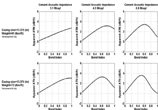
Figure 5: Modeled apparent attenuation vs. bond index for an 8.25-in. tool inside 13.375-in. casing.
