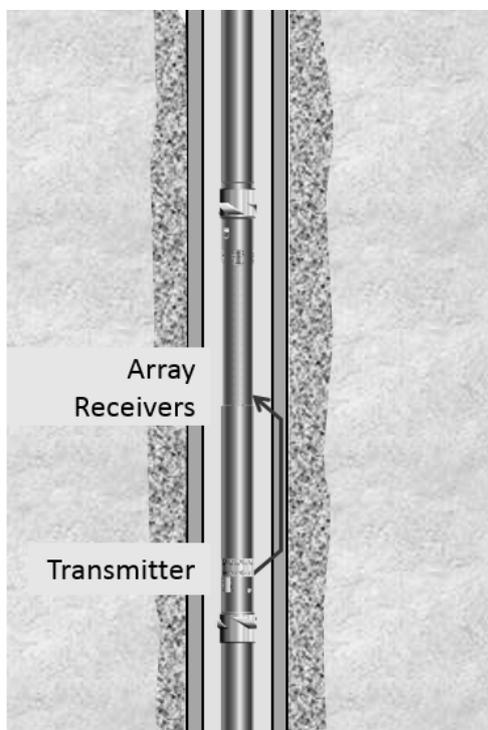
Figure 1: An LWD sonic tool is shown above inside casing. The signal which travels in the casing and arrives at the array receivers contains information which can be used to determine how well the cement is bonded to the casing.
