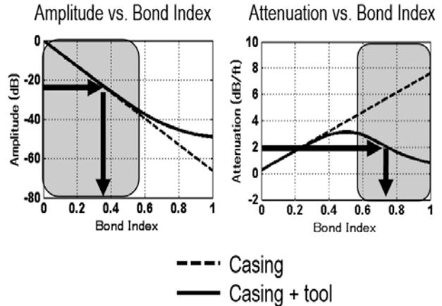
Figure 3: Bond index conversions for amplitude (left) and attenuation (right). Amplitude is used for lower bonding conditions while attenuation is used in higher bonding conditions,
