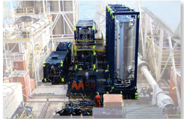
A compact surface well test setup used offshore Brazil.
