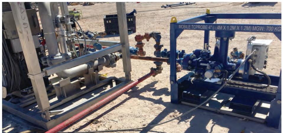
The AquaWatcher Surface sensor is installed in series with PhaseTester equipment for salinity determination in real time.
