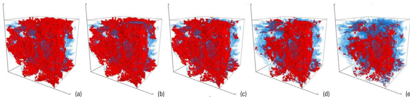
3D phase saturations at selected time intervals progressing from (a) to (e) during steady-state flooding of a sample. Water is blue and oil is red in the transparent digital rock.
