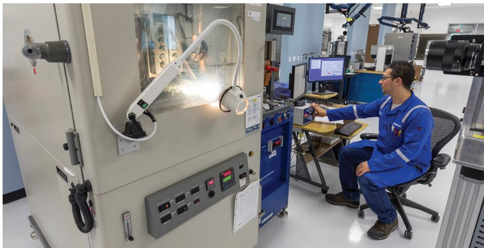
*The modular design of the single PVT system streamlines employing various configurations for conducting a wide variety of fluid phase behavior investigations.*
