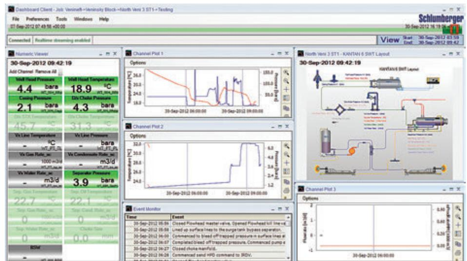
TestingManager platform visualization showing real-time PVT measurements, reservoir data, and events during the Venineft test operation.
