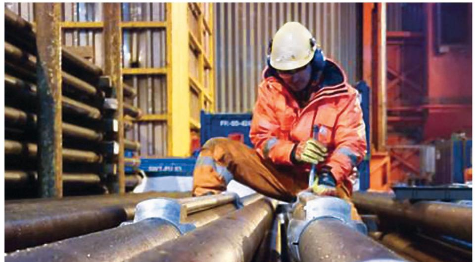
Schlumberger engineer preparing the wireless-enabled DST toolstring to run in hole.
