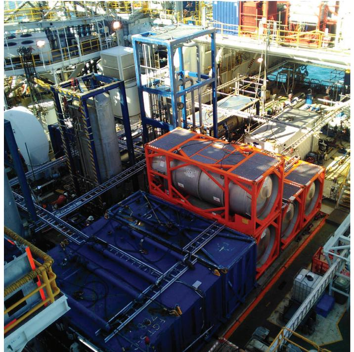
*Facility to treat contaminated condensate at the surface before reinjecting back into the production pipeline, offshore New Zealand.*
