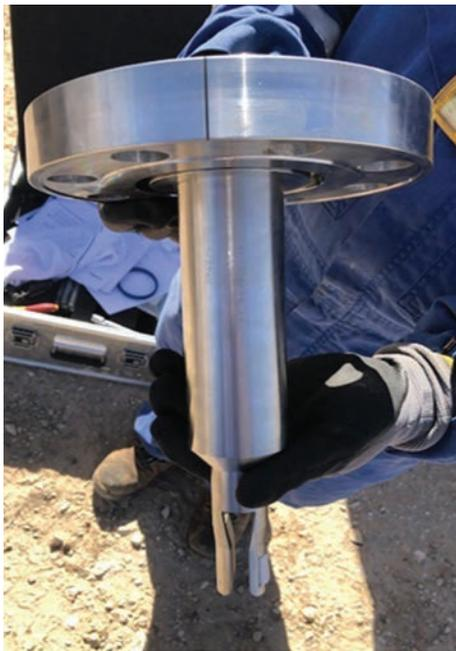
*The lightweight and compact low-rate extender is easy to install in existing or new Vx Spectra surface multiphase flowmeters.*
