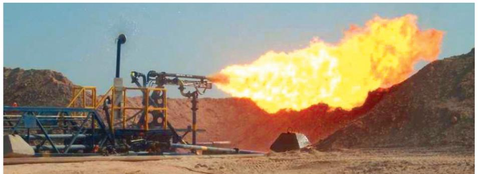
*EverGreen burner with monojet configuration produced no smoke or fallout while burning heavy oil.*
