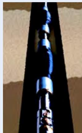
**MDT packers are inflated to isolate a reservoir zone for fluid sampling and pressure measurements.**
