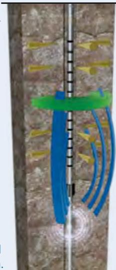
with 5 transmitters and 104 receivers, with a unique dipole source design that enables it to be fired in either pulse or "chirp" mode. Slowness identification using the Sonic Scanner aided the RIL-Schlumberger drilling team in denoting optimal pretest/sampling point selection, thereby saving considerably in nonproductive rig time. The tool also proved beneficial for evaluating radial acoustic behavior behind cemented casing intervals.
