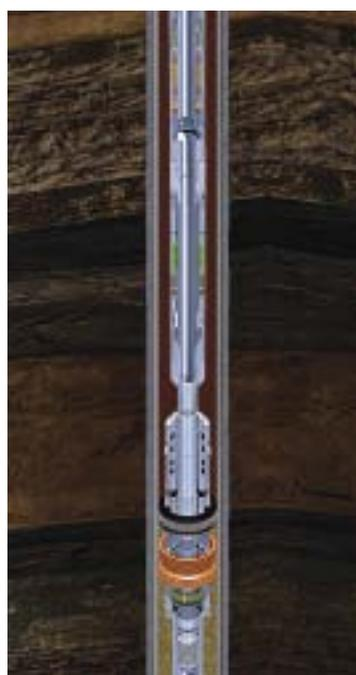
**TEST MATCH:** Enabled by Muzic wireless telemetry, the Quartet downhole reservoir testing system provides data in real time for validation.
