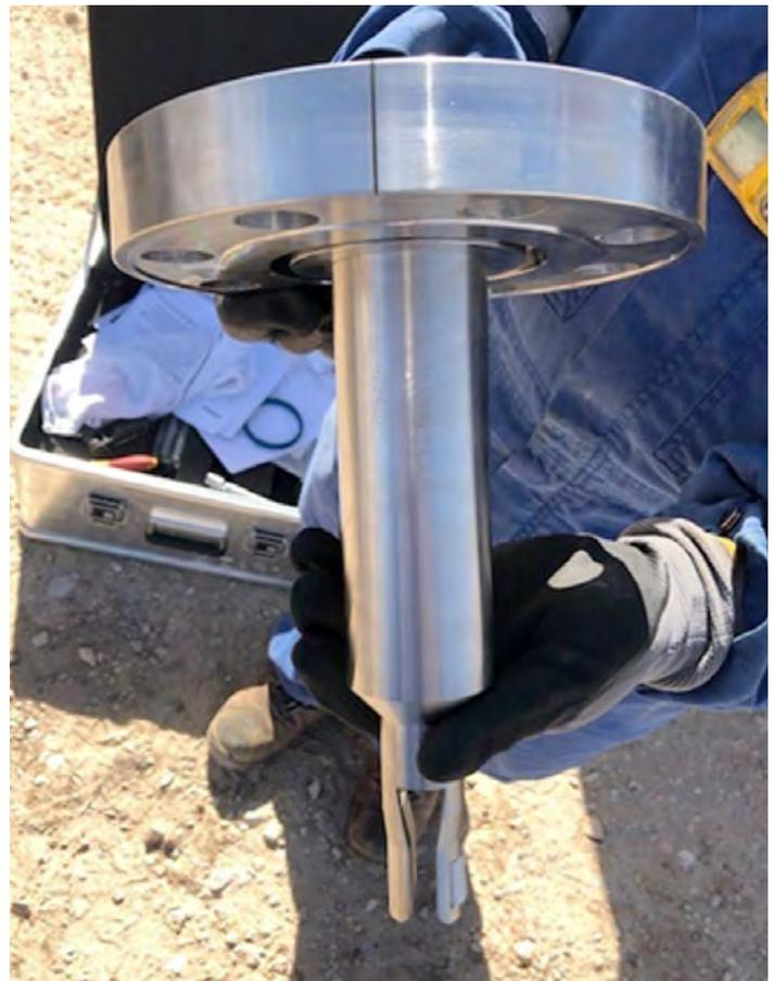
FIGURE 1. The low-rate extender insert is installed across the venturi section of a multiphase surface flowmeter. (Source: Schlumberger)
