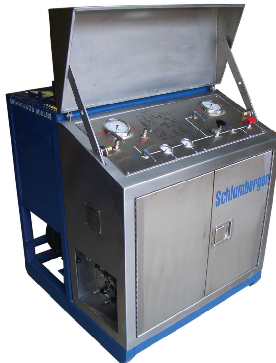
Well test ESD system.
