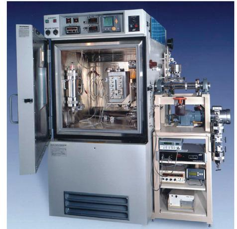
*Phase behavior PVT system for the study of vapor-liquid-aqueous-solid equilibria for gas condensate and oil systems.*
